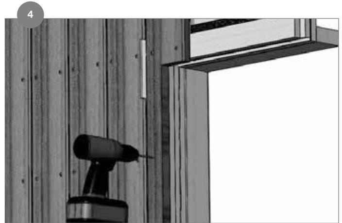
Notch boards for openings in the wall. Always pre-drill holes in widths 3 in. or under, and secure with one #8 x 2 1/2 in. composite deck screw.
