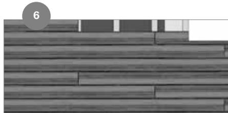
As courses are added, stagger butt joints in a consistent "stair step" fashion for best results. Never allow a butt joint directly over or under an opening in the wall. Stacked butt joints are permitted, but require special care in gapping. At butt joints, fasteners must be installed perpendicular to the board. Angling fasteners is not permitted.
